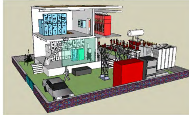
Compact 33 kV Distribution Station
