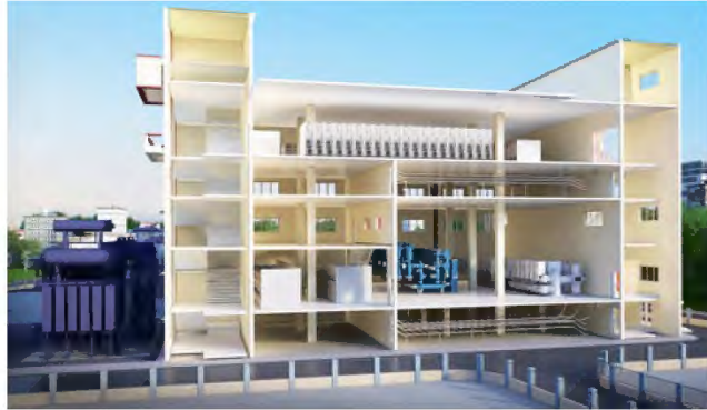
Integrated SS at New Cossipore with 220, 132 & 33 kV GIS
